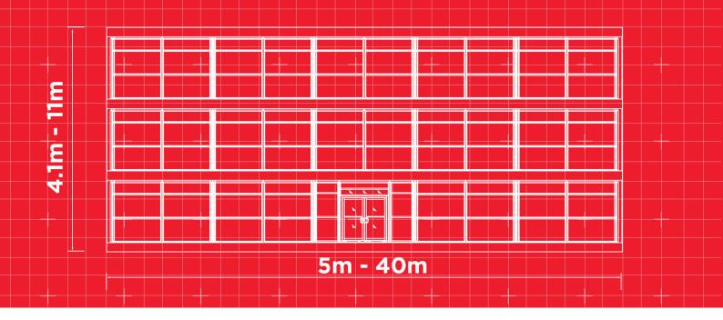
Size: Levels: G + 35x5m, 5x7.5m **Level Height:** 4.01m Walling: Seamless Glass, Glass Panels, ABS Panels, **Internal Height:** 3.13m **PU Panels** Wind Loading: 160km/h Terrace: 2.5m Cantilever Balcony **Design Codes: Temp. / Permanent use Wall Bracing: Not Required**
